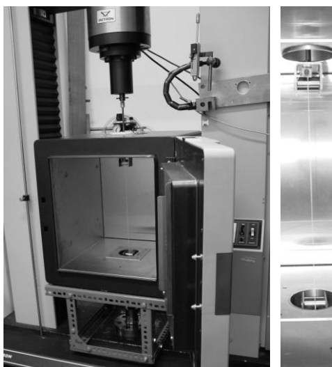
Figure 1. Experimental set-up for tensile and SIM tests
