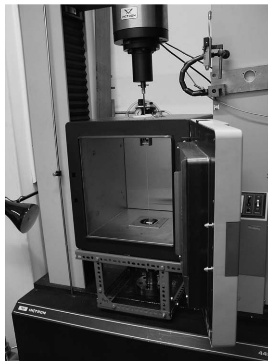
Figure 6 Experimental set-up for tensile and SIM tests.
