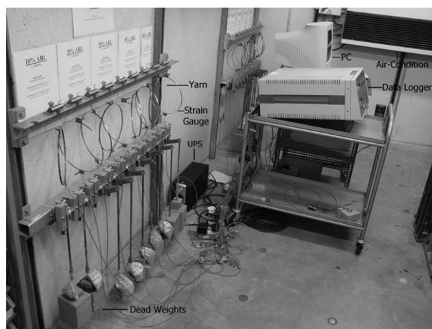
Figure 5 Experimental set-up for CCT tests.
